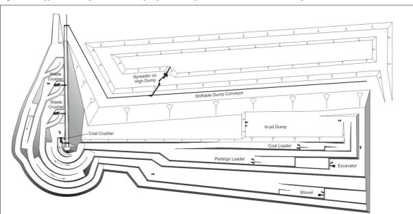
Figure 6 – Typical Pit Layout for A Deep Open Cut Operation in the Hunter Valley.
