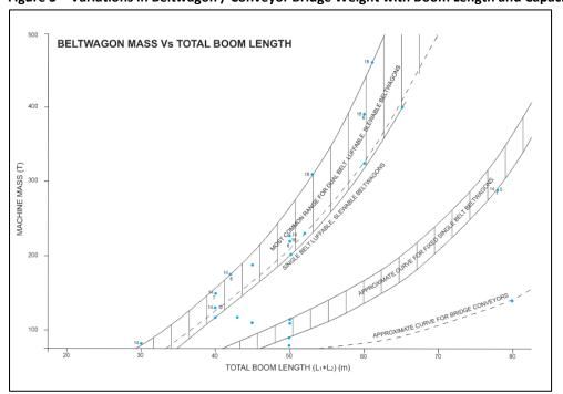
Figure 3 – Variations in Beltwagon / Conveyor Bridge Weight with Boom Length and Capacity
