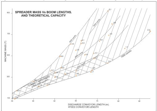
Figure 4 - Variations in Spreader Weight with Discharge Boom Length and Capacity
